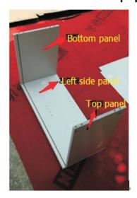
Fix the left panel and the bottom panel with eccentric wheel
