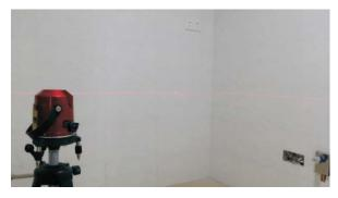
Confirm the position of each cabinet according to the drawing.
