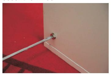
5.6 Connect the right panel to the bottom panel and top panel, like the picture shows
