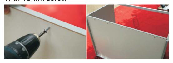
6.12 Fix the adjustable leg with 15mm screw
