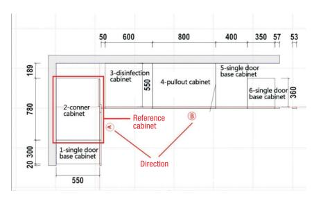
3.2 Confirm the "Installation Direction (from which direction to which)" according to the drawing.
